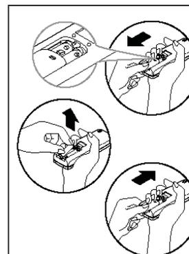
The remote controller is powered by two dry batteries(R03/LR03X2) housed in the rear part and protected by a cover.
